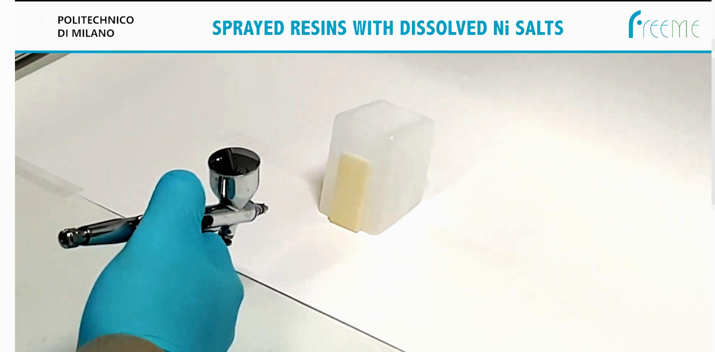
Polimi: Sprayed Resins
