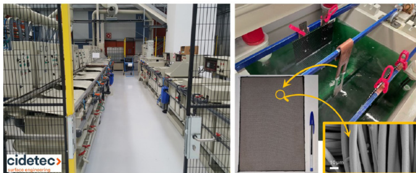
Fig. 1 CIDETEC's pilot line (left) and the produced 450 cm 2 PEM WE Ni-based porous electrodes (right).
